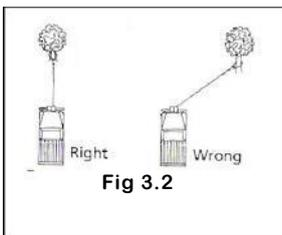
**CAUTION** Do not winch from an acute angle as the wire rope will pile up on one side of the drum causing damage to wire rope and the winch. Fig 3.2
